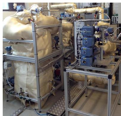
Large-scale ejector based recirculation subsystem
