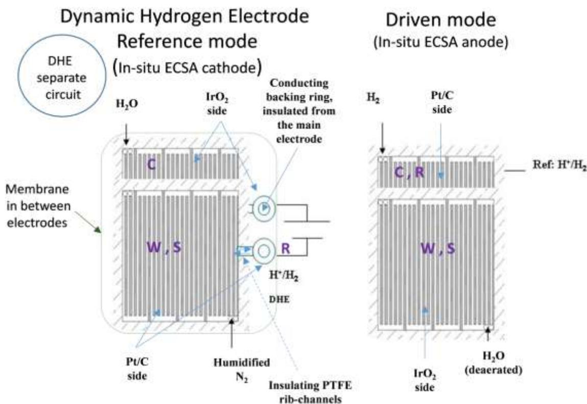
**Figure 1** PEMWE configurations for the *in-situ* measurement of the ECSA by CV of the cathode in DHE mode (left) and of the anode in driven mode (right); the arrows (solid blue) indicate the presence of Pt/C and IrO<sub>2</sub> catalyst on their respective electrodes; the capital letters C, R, S and W refer to counter electrode, reference electrode, sense electrode and working electrode, respectively (adapted from [7]).
