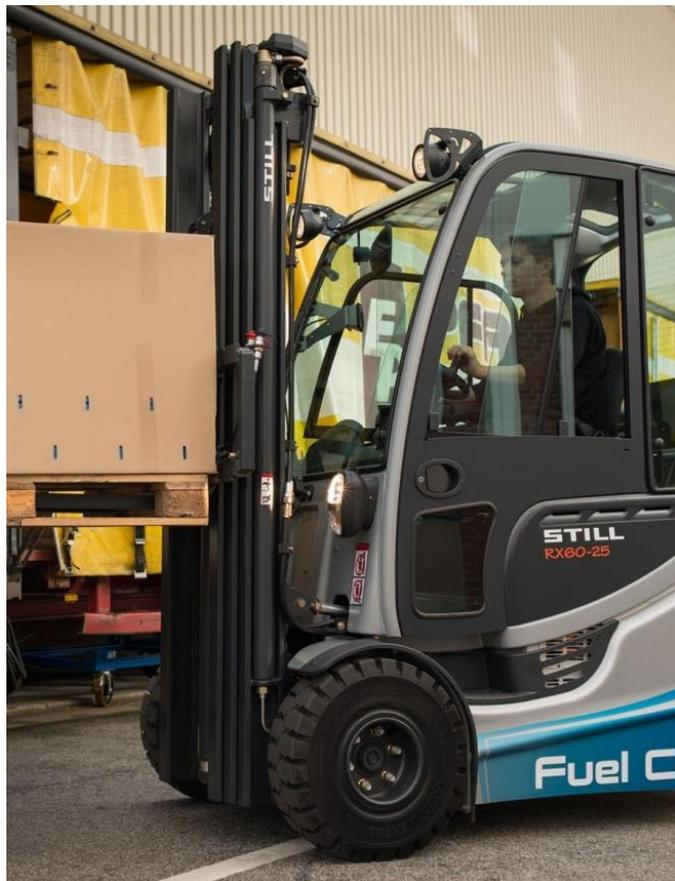
**Brief description:** Fuel cell material-handling equipment, e.g. forklift trucks, use compressed hydrogen gas as a fuel to generate electric power via an energy converter (fuel cell); the produced electricity powers an electric motor as well as the forklift
