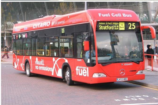
**Brief description:** Fuel cell electric buses built on a conventional chassis (12-18m) use compressed hydrogen gas as a fuel to generate electricity via the fuel cell (FC dominant powertrains). Other hybrid vehicles e.g. with plug-in batteries or FCH range extenders (larger battery, smaller FC) as well as minibuses are pursued as well
