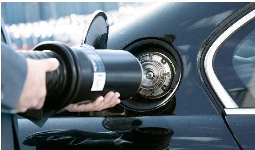
Figure 4 Filling coupling for liquid hydrogen, (Hy Approval project, 2008).
