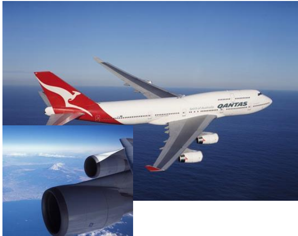
A Qantas Boeing 747-400 powered by the GE CF6-80C2 (source: www.geaviation.com )
